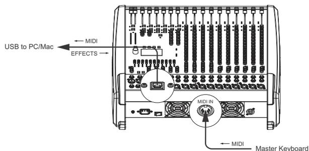
The PowerMate offers similar options for the creation of sound effects. The PC serves as an external, extremely powerful multi-effects unit. Since the signal is fed from one or both AUX ways, the operation during mixing becomes as simple as using the internal effects of the PowerMate. The AUX ways should be switched to post-mode. The effect signal generated in the PC is again added to the overall mix via USB stereo channels 1-2 and 3-4. The stereo channel faders serve as FX-return controls.
