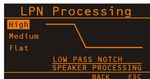
Turn the MENU/ENTER rotary encoder to select the preferred LPN filter setting, see the following table for details. Press the MENU/ENTER rotary encoder to apply the selected setting. Pressing the BACK function key returns to the menu. Pressing the ESC function key discards all changes and returns to effect mode.
