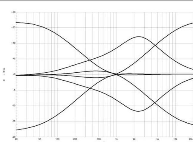
The EQ section of the STEREO channels is designed in a way that HI and LO controls provide a degree of control that is equally adequate for LINE level inputs and microphones. The MID control is active in a comparably wide frequency band around 2.4 kHz. With most microphones this is the critical range, where a slight attenuation offers excellent results.
