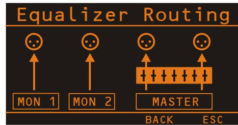
Turn the MENU/ENTER rotary encoder to change the routing of the Graphic Equalizer. Press the MENU/ENTER rotary encoder to apply the selected routing. Pressing the BACK function key returns to the menu. Pressing the ESC function key discards all changes and returns to effect mode.
