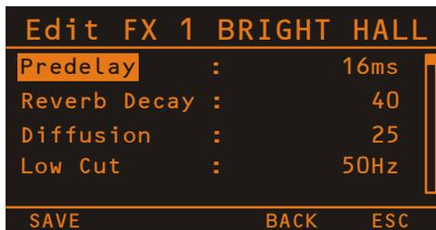
Turn the MENU/ENTER rotary encoder to highlight an entry in the left column of the Edit FX Menu. Press the MENU/ENTER rotary encoder to select the corresponding value in the right column. Now turn the MENU/ENTER rotary encoder to edit the value. Press the MENU/ENTER rotary encoder again to return to the left column. Press the SAVE function key to store the edited effect as an user preset. The FX User Presets dialog appears.
