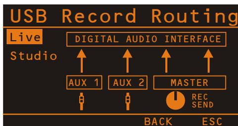
Turn the MENU/ENTER rotary encoder to select the assignment of PowerMate busses to channels USB 1 to 4 of the DIGITAL AUDIO INTERFACE. Following table lists the available assignments. Press the MENU/ENTER rotary encoder to apply the selected assignment. Pressing the BACK function key returns to the menu. Pressing the ESC function key discards all changes and returns to effect mode.
