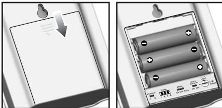
**NOTE** Replace the batteries whenever the low battery icon
