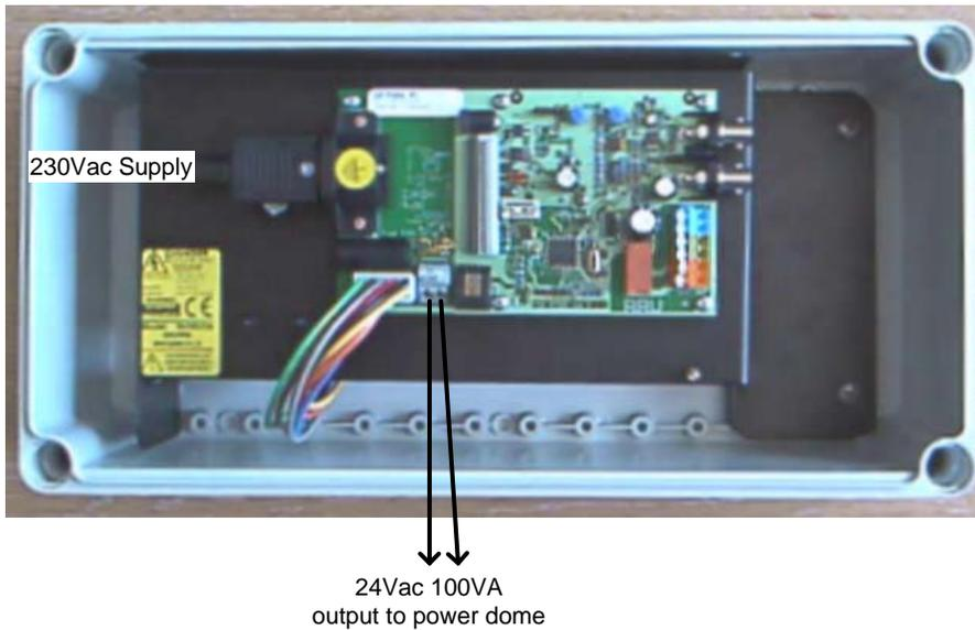
**Important!** When operating the unit from 24Vac, the fuse from the 230Vac connector fuse holder must be removed. No connections must be made to this connector, as it will have 230Vac across the L & N terminals.
