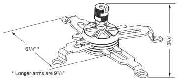
Please Note: This is total height of Universal Projector Bracket. Once attached, Universal Bracket actually adds a minimum of 3" to overall mount size.
