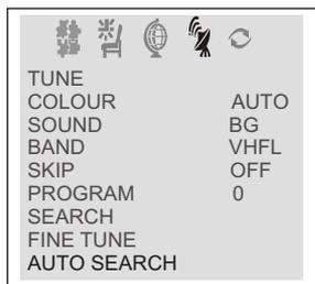
3 Press the VOL+ button to ensure automatic search function operates. All channels now playing program will be automatically preset in order . After the search has finished, the first program number will display on the screen.
