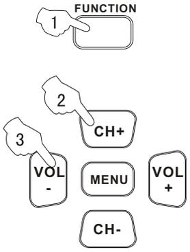
1 Press the FUNCTION menu button, till the FUNCTION menu shown on the right display on the screen.
