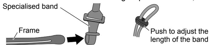
When the end of the specialised band is straightened, form a loop at the end of the band, and fix the twisted part.
