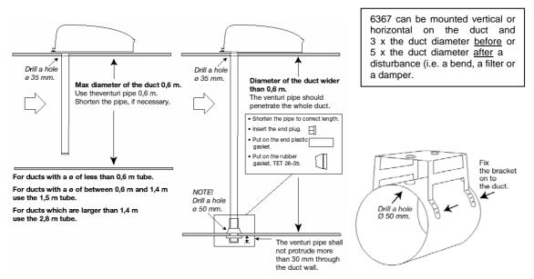
*Left:* How to suit the pipe to different widths of the ventilation duct. *Right:* The Bracket 6372. Attached with each Duct detector chamber are detailed mounting and installation instructions.
