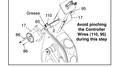
Connect the Left Handlebar Wire (108) to the Left Controller Wire (110). Insert the excess wire into the Left Handlebar (8).
