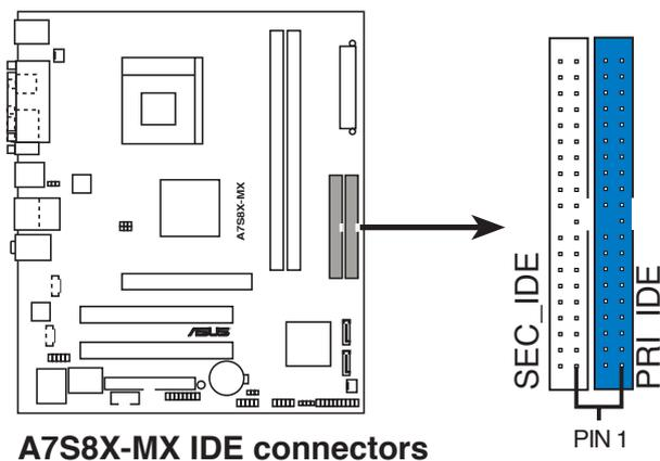
**NOTE:** Orient the red markings (usually zigzag) on the IDE ribbon cable to PIN 1.
