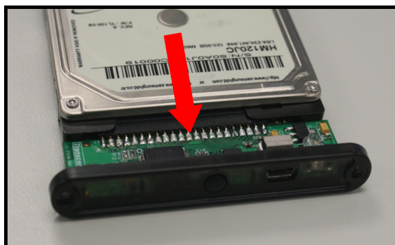
Figure 4. Connect the hard drive to the IDE adapter
