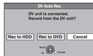
Press [◀, ▶] to select "Rec to HDD" or "Rec to DVD" and press [OK].
