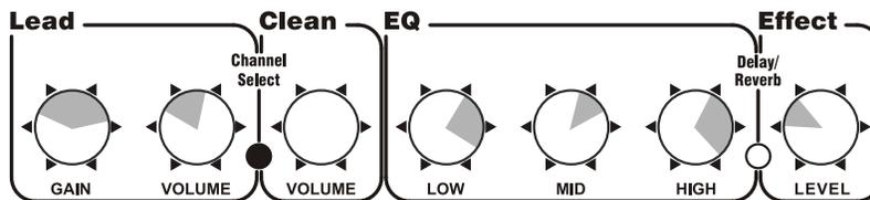
**Medium-Gain Rock and Blues** - this setting is particularly useful in blues or classic rock songs. It is good for leads as well as rhythm parts. It is also useful for power chords. You need to switch to the lead channel to make these settings work. Blues, depending on the guitar you use, usually adds treble but with more midrange and a "fat" bottom end. Adjust the gain control to the amount of distortion you desire. Blues often has a reverb trail on the notes. Adjust to taste.
