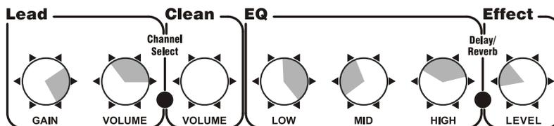
**Heavy Metal/Maximum Crunch** - this setting is a good starting point for the "notched-out middle" sounds associated with metal and heavy alternative sounds. Adjust the Treble, Lows, and Delay to taste. Usually, for a rhythm tone, you want to have more lower end and less for leads. Distortion is an integral part of this style of music, so crank up the Gain.
