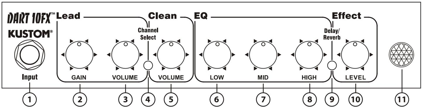
**1.) Guitar Input Jack** -This is a 1/4" 2-conductor input jack for plugging in your instrument. It is intended for guitars but will accept other instruments as well.
