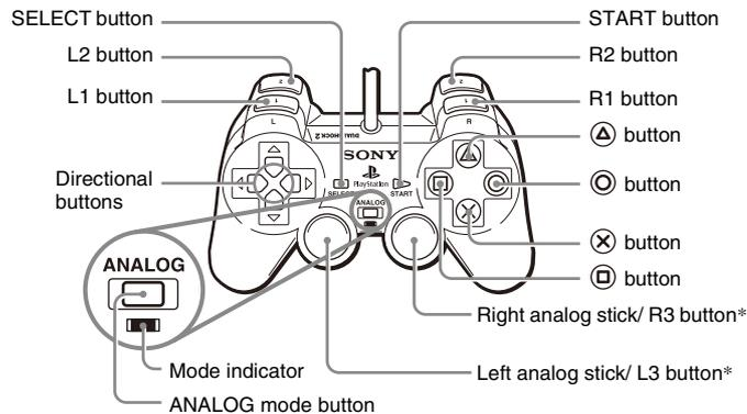
\* The left and right analog sticks, or the L3 and R3 buttons, function only in analog mode (indicator: red).
