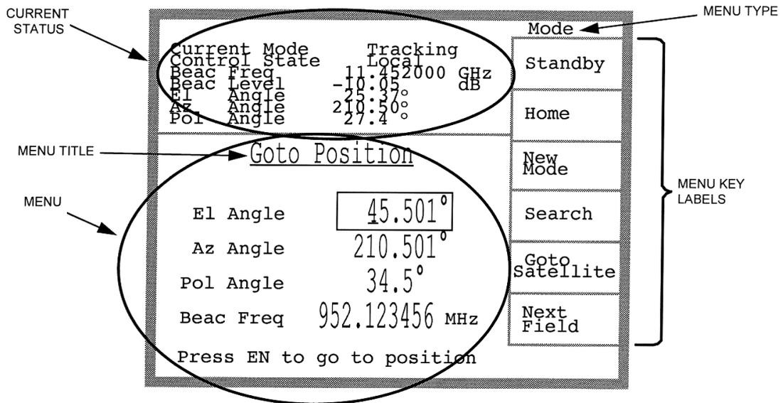
A typical menu display screen is shown above. In this example it is the "Goto Position" used to drive the antenna to a particular pointing angle.
