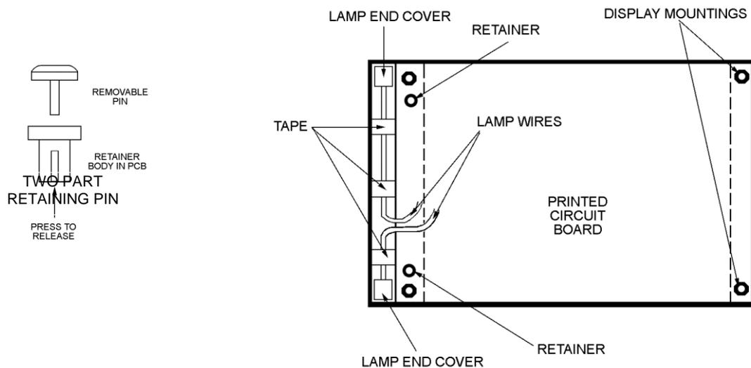
Turn the display face up. Remove the retainer pins. Remove the metal cover.
