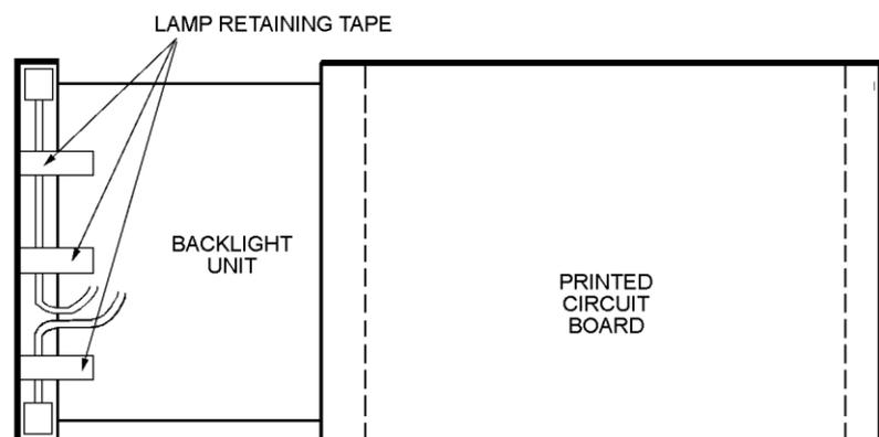
Remove the three tapes which secure the lamp reflector. Remove the lamp and wire assembly.
