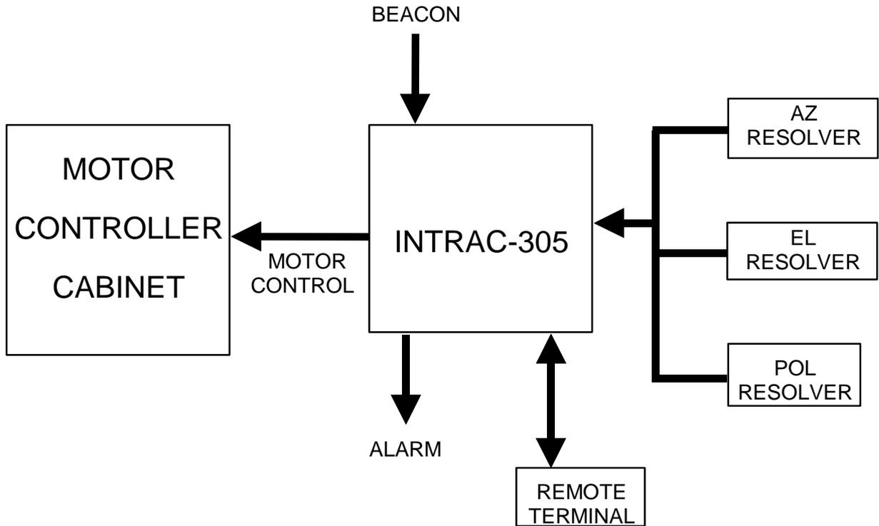
All connections to the INTRAC-305 are made via its rear panel. The following connectors are available :-
