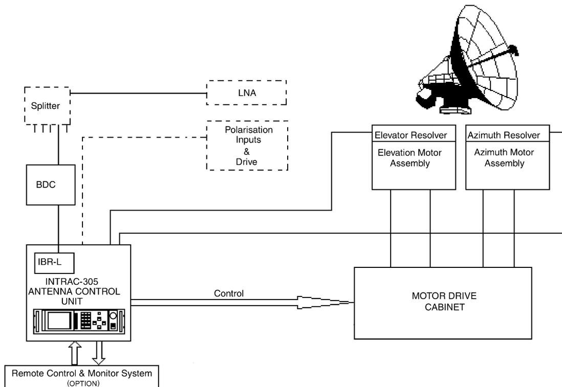
The antenna position resolvers provide direction information to the INTRAC. The IBR-L (beacon receiver) provides tracking signal strength. (A signal strength derived dc voltage from an external receiver may be used in place of the Advantech AMT IBR-L)
