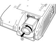
Remove the lens cap (on the back) from the replacement lens.
