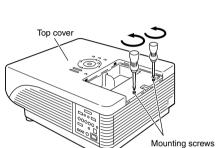
Remove the mounting screws of
