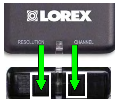
Figure 5.0 Hold the CHANNEL button to pair additional cameras
