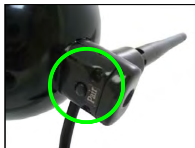
Figure 5.1 Pair button underneath antenna
