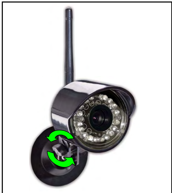
Figure 1.1 Attach the camera to the stand
