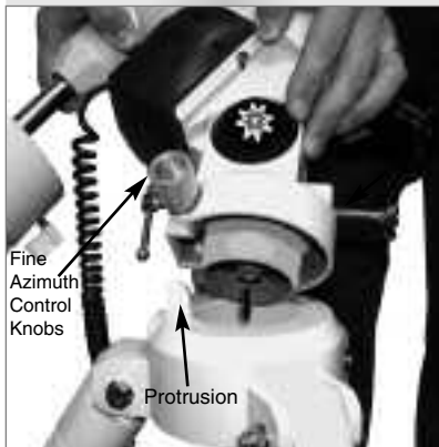
Fig. 4: Attach the mount to the tripod.
