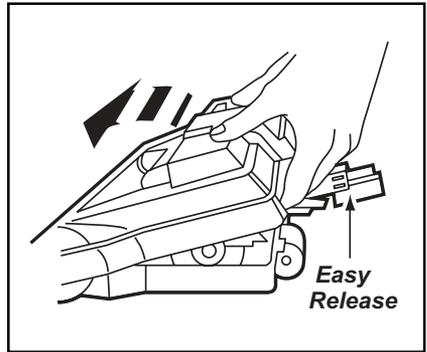
3. Turn Electroglide Powerhead over. To remove cover, insert screwdriver at cover tabs on both sides and twist to release tabs.
