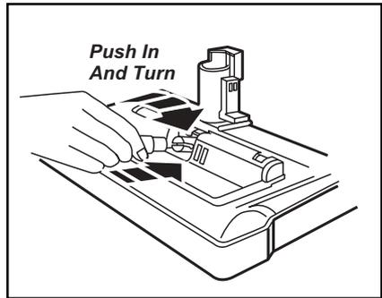
3. Push in and turn bulb counter clockwise to remove.
