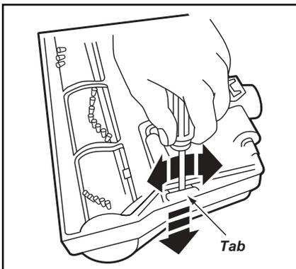
5. Carefully insert and twist screwdriver at each brush support to free brush from base.
