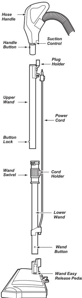
1. Connect the upper and lower wand sections. (The wand swivel is located on the lower wand.)
