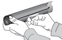
4. Grasp the lock lever and place the left side of the toner cartridge into the toner well, under the tab.
