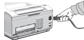
3. Turn the printer on. It takes about 10 seconds for the printer to initialize, warm up, and display the **ON-LINE** message, indicating the printer is ready to receive data.
