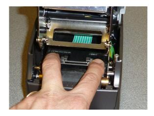
Step 2: Place media guide in printer behind the platen roller with index sensor centered.
