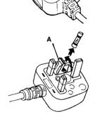
Type 2: Prise up the hinged fuse cover (A) as shown.
