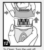
unit by squeezing both sides of the disc cover and pulling up.
