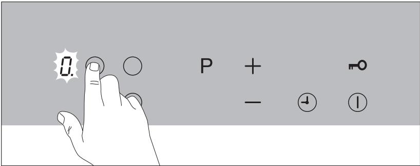
2. With the ⊕ or ⊖ sensor fields select heat setting [9]. Stop briefly and touch the ⊕ sensor field again.
