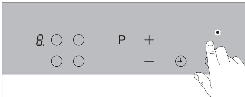
2. To release the lock touch the "Lock" sensor field again continuously until the control indicator goes out.
