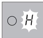
Even after the cooking zone has been switched off, the residual heat indicator only goes out when the cooking zone is cold.
