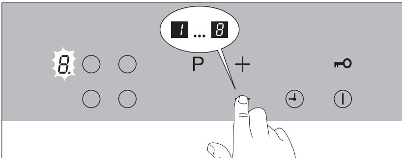
After 5 seconds, **A** appears in the display again instead of heat setting selected for further cooking. The heat setting is displayed again after the heating-up time has ended.
