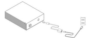
2. Attach the USB 2.0 cable to the drive.
