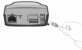
**TIP:** You can confirm power source is supplied from the LED indicators label Power on the SkyIPCam310 is illuminated.
