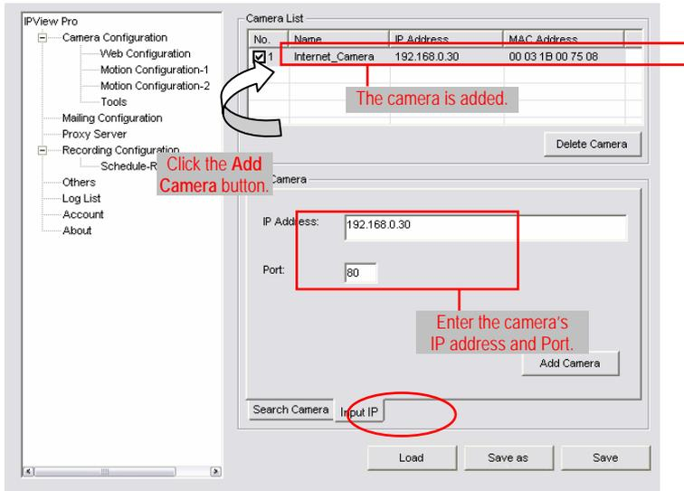
5. Enter the camera's IP address (you can get this from the AirLink101 camera setup wizard application) and Port (default: 80), and then click **Add Camera**.
