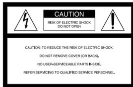
This symbol is intended to alert the user to the presence of uninsulated "Dangerous voltage" within the product's enclosure that may be of sufficient magnitude to constitute a risk of electric shock to persons.
