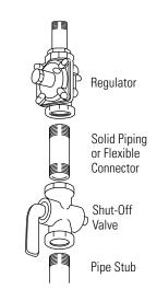
IMPORTANT: Disconnect the cooktop and the individual shut-off valve from the gas supply piping system during any pressure testing of that system at test pressures greater than 1/2 psig. Isolate the cooktop from the gas supply piping system by closing the individual manual shut-off valve to the cooktop during any pressure testing of the gas supply piping system at test pressures equal to or less than 1/2 psig.
