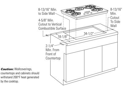
Measure carefully when cutting countertop. Make sure sides of opening are parallel and rear and front cuts are exactly perpendicular to sides.
