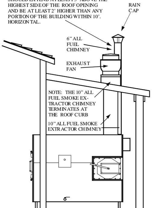
NOTE: THE 10" ALL FUEL SMOKE EXTRACTOR CHIMNEY TERMINATES AT THE ROOF CURB
