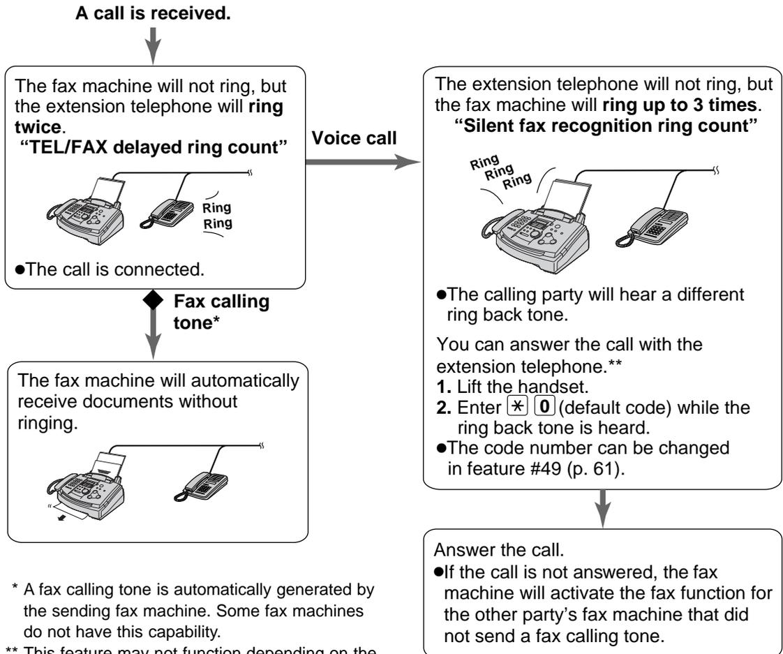
\* A fax calling tone is automatically generated by the sending fax machine. Some fax machines do not have this capability.
