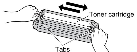
**11** Install the drum and toner unit by holding the tabs.
