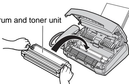
**12** Close the front cover, until locked, by pushing down on both sides.
