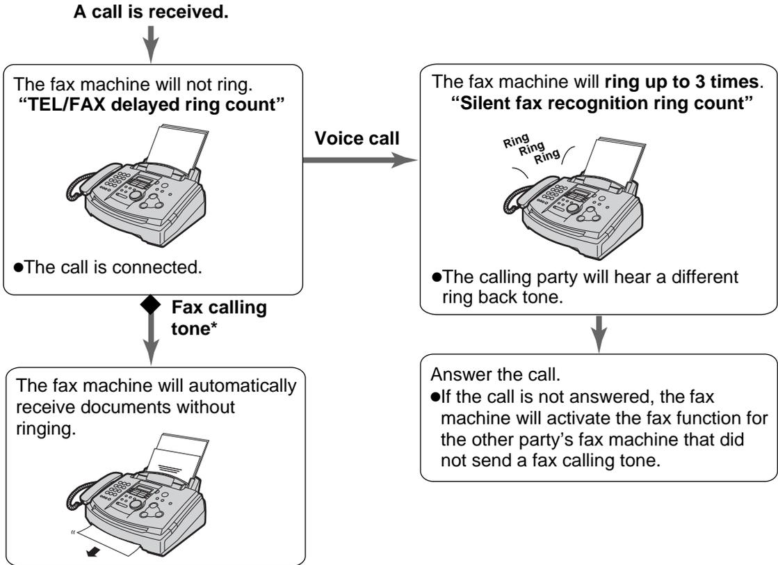
\* A fax calling tone is automatically generated by the sending fax machine. Some fax machines do not have this capability.
