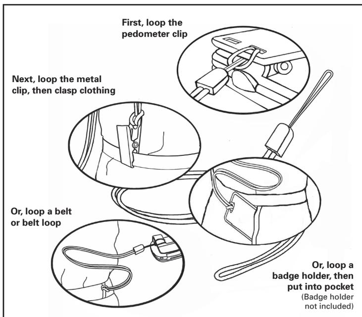
**Attaching the Leash:** Attach the pedometer to the leash by looping the leash around the pedometer belt clip. Next, clasp the waistband of your clothing with the attached metal clip. You can also use a safety pin to fasten the leash to your clothing, or loop the leash through your belt or belt loop.
