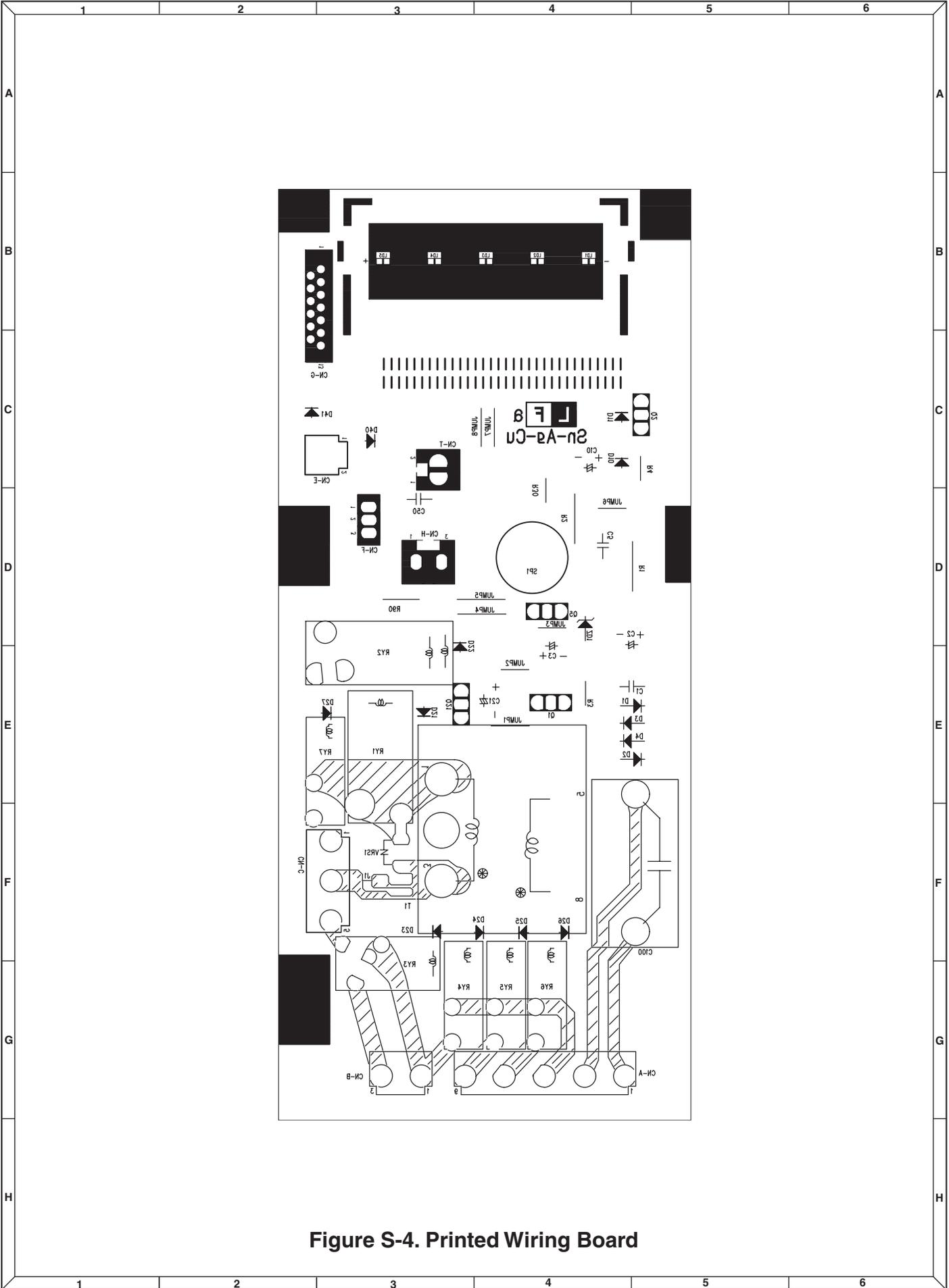
Figure S-4. Printed Wiring Board
