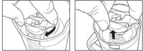
**Note:** To reassemble, reverse the above procedures and make sure the valve is locked in place before blending again. The small arrow on the valve front will line up with the small arrow on the jar bottom where the locked padlock picture is shown. If the valve is not properly locked in place, ingredients will leak from the drain hole in the bottom of the jar.
