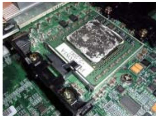
3. Push the lever back down and fix a processor.
