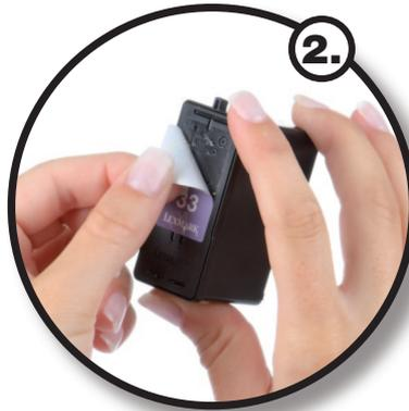
First remove the label from the upper side of the cartridge and bore refilling holes. To do so, use the supplied tool to enlarge the 3 existing openings.
