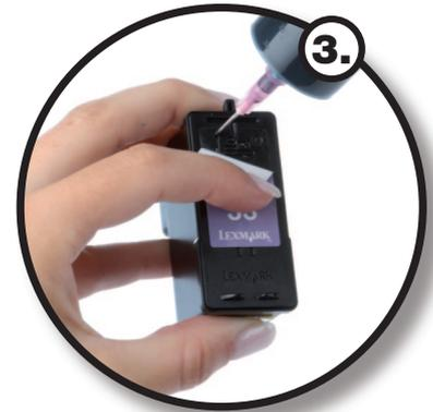
Now insert the syringe inclined into each opening. Slowly and carefully squeeze the ink into each ink chamber, until just under the openings. If some ink emerged from the nozzles, simply draw up a small quantity of ink from the chamber into the syringe. To make sure that you inject the right colour into the correspondent colour chamber while refilling, start to identify each colour chamber, inserting a toothpick through the openings. Replace the label afterwards.
