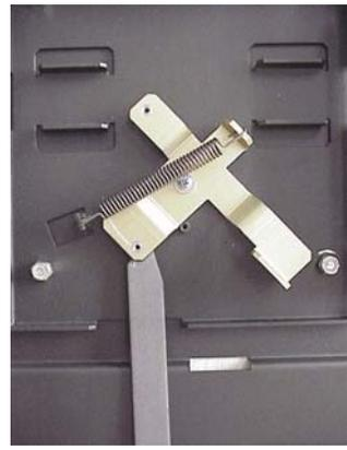
**Unlocking from the bottom:** Slide the tool in from the bottom, keeping the open side of the hook to the left, as shown. Catch the lock and pull down.
