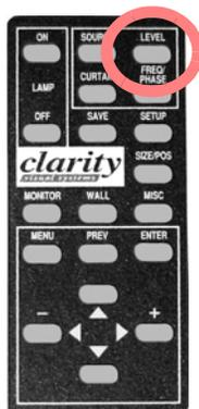
LEVEL key opens the Input Levels menu directly
