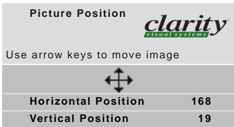
The numbers for Horizontal and Vertical Position refer to the number of pixels from sync to the first displayed pixel. These numbers get smaller as the picture moves up and to the left.
