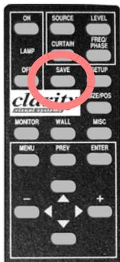
Pressing the SAVE key opens the Recall menu. A second press opens the Save menu.
