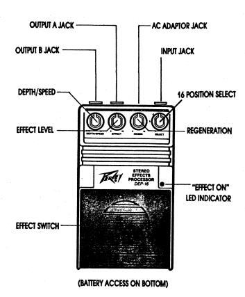
**INPUT JACK:** Used as a signal input to the effects unit. This jack also acts as a power switch for the unit when an instrument is plugged in. When the effect is not in use, the instrument should be disconnected from this jack to maximize battery life.
