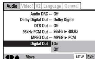
Settings: **On** (Digital bitstream is output) (Factory setting)
