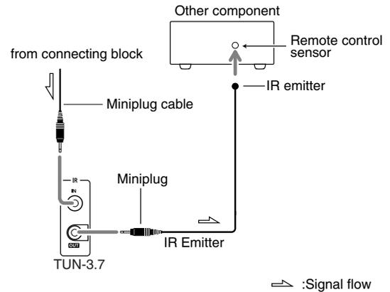
Only remote controller signals received by the TUN-3.7's IR IN are fed through to the IR OUT. Signals picked up by the TUN-3.7's remote control sensor are not output.
