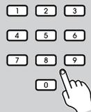
For example, to tune into an FM station at 87.5 MHz, press [8], [7], and [5].
