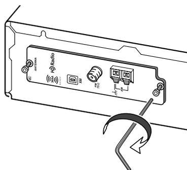
Be sure to fully tighten the screws. If they are loose, the ground connection between the board and the TUN-3.7 may be inadequate, resulting in noise or failure.
