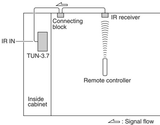
Connect the IR receiver to the TUN-3.7 as shown below.
