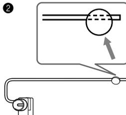
Affix the antenna with a thumbtack. (Do not push the thumbtack *through* the antenna.)
