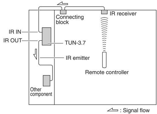
Connect the IR emitter to the TUN-3.7's IR OUT, and place the IR emitter in front of the other component's remote control sensor (usually located on its front panel), as shown below. See the instructions supplied with the IR emitter.
