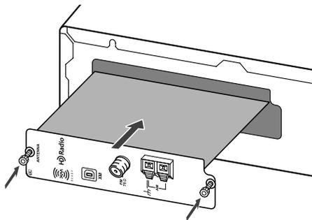
When the board meets the internal connector, apply a little more pressure so that the board plugs fully into the connector. Make sure the board's panel is flush with the TUN-3.7's rear panel.
