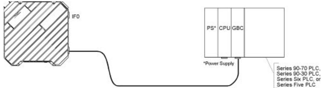
Figure 3 - 3. PLC/Panel Connection
