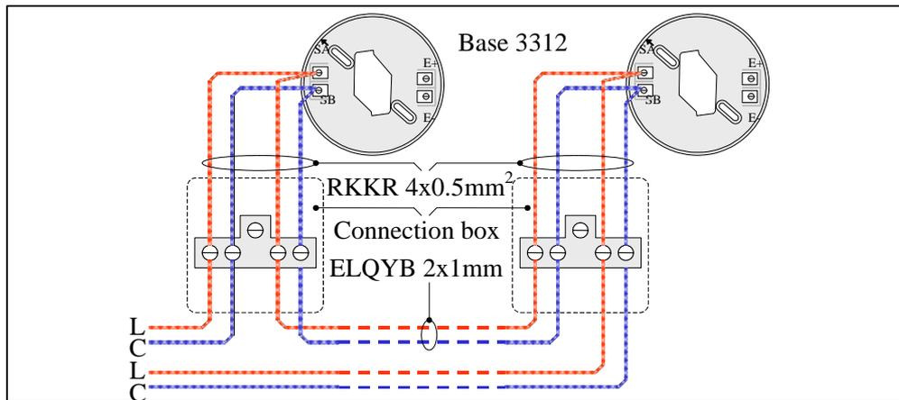
Example showing how to connect the Analog base 3312.
