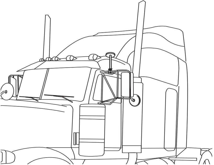
*Figure 1. The TERK SIR4-Truck Satellite Radio Antenna is shown installed on the horizontal driver's side mirror support of a long-haul truck.*
