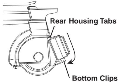
Insert upper filter corner tabs firmly under rear housing tabs and pivot filter down until bottom clips on filter click securely into place on the cleaner.
