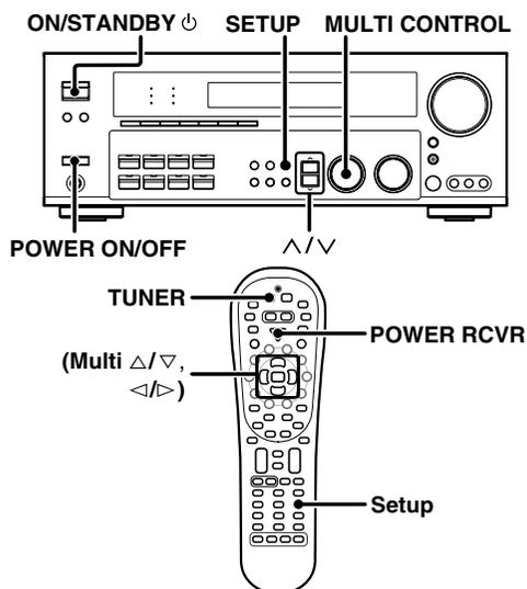
**1** Turn on the power to this receiver by pressing the **POWER ON/OFF** and **ON/STANDBY** key or **POWER RCVR** key.
