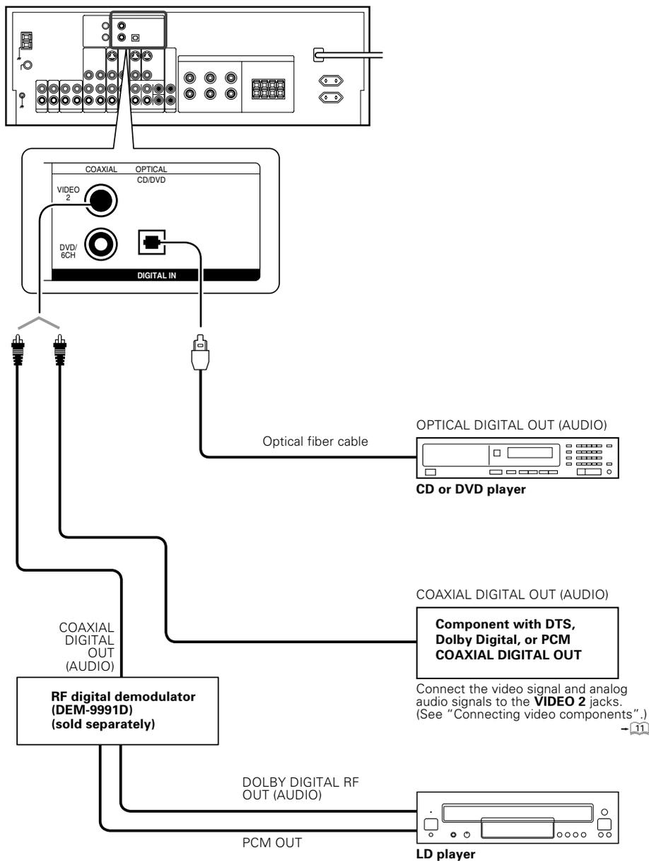
To connect an LD player with a DIGITAL RF OUT, connect the LD player to the KENWOOD RF digital demodulator (DEM-9991D). Next, connect the DIGITAL OUT jacks of the demodulator to the DIGITAL IN jacks of the receiver. Connect the video signal and analog audio signals to the VIDEO 2 jacks. (See "Connecting video components".)
