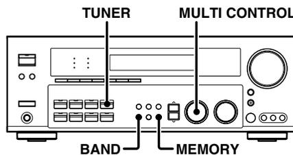
1 Press the **TUNER** key to enter tuner mode.
