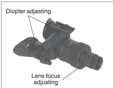
To focus the NVG-7, first you will need to adjust the diopter. Simply turn the diopter clockwise until it stops. Then, while looking through the diopter at an object, slowly turn the diopter back counter clockwise until the grain in the image is sharp.
