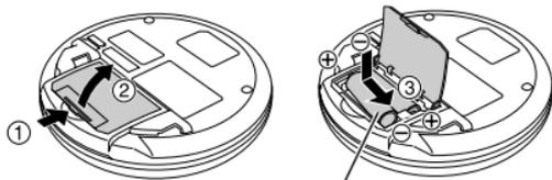
Two "LR6" alkaline batteries.
