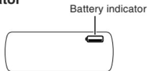
This indicator appears when the batteries are almost out of power. Power will be cut off a short while later.
