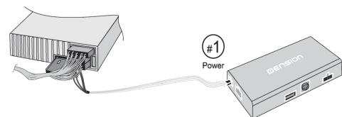
Plug the power cable lead to the Gateway Lite D2B.
