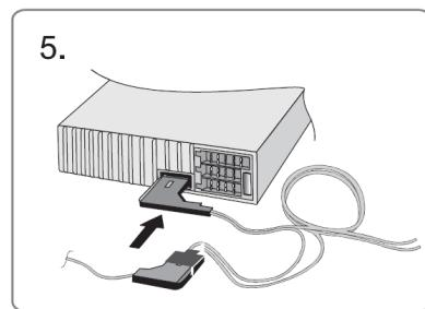
(6.) Plug the last flying connector of your optical harness to the Gateway Lite D2B interface, with this step you are connected to the D2B optical ring.
