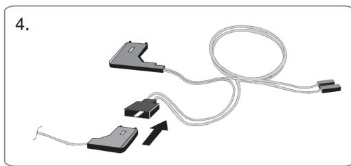
(5.) Connect the #21/22 A connector to the back of head unit.
