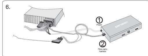
Finally connect each cable according to the numbers in the first picture. Lead away the cables where the devices will be placed. (E.g the glove compartment or the center console).
