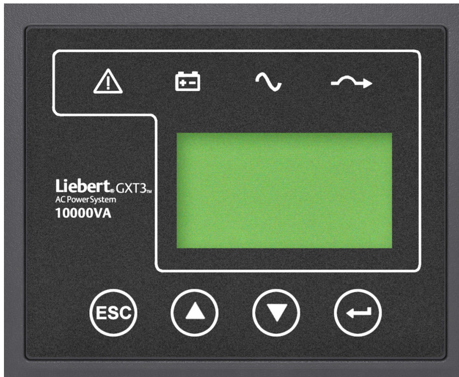
Figure 1 Liebert GXT3-10000T220 control panel
