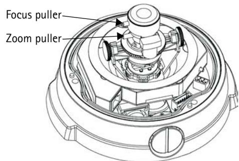
**Note:** The DC-Iris should always be disabled while focusing the camera. This opens the iris to its maximum, which gives the smallest depth of field and thus the best conditions for correct focusing. When the focus is set with this method it will then be maintained in any light conditions.
