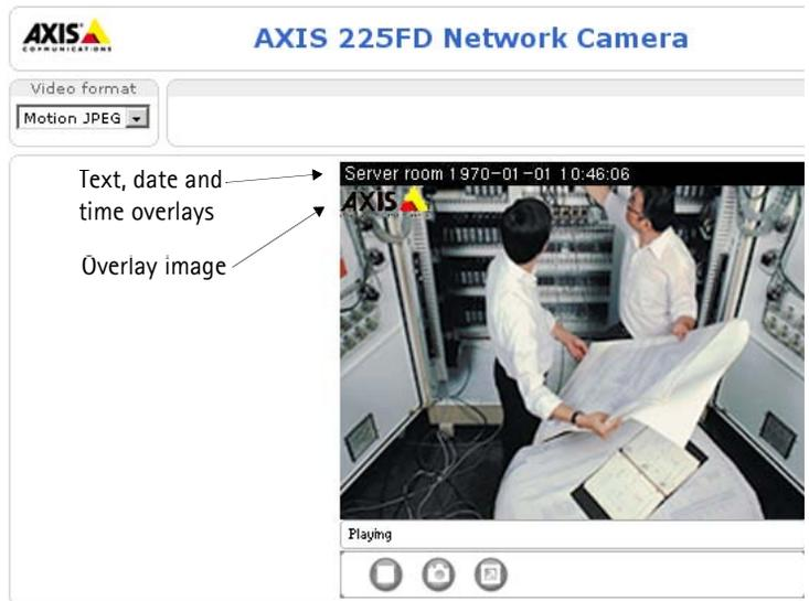
The difference between an overlay and a privacy mask is that a privacy mask cannot be bypassed by accessing the video stream with the help of the AXIS HTTP API, whereas an overlay can.
