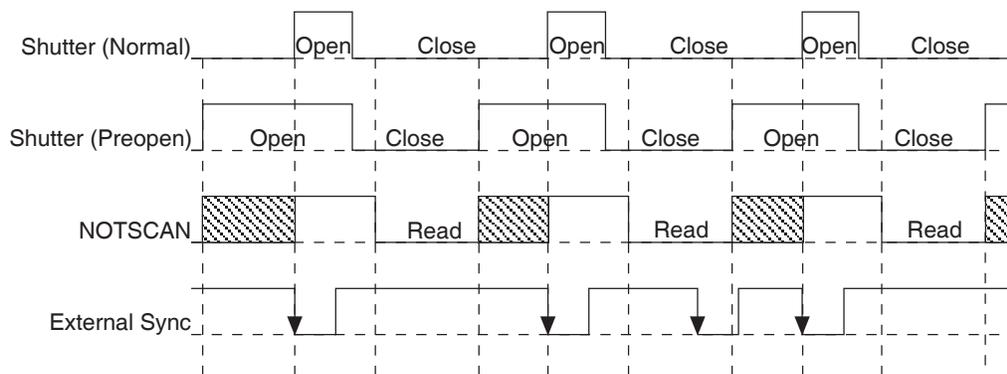
Figure 15. Continuous Cleans Timing Diagram
