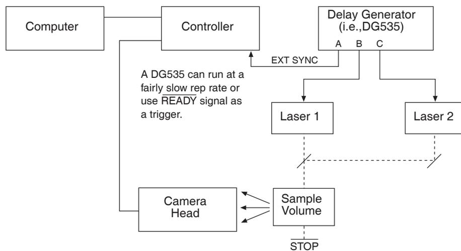
Figure 55. Setup for IEC Experiment with Two Lasers
