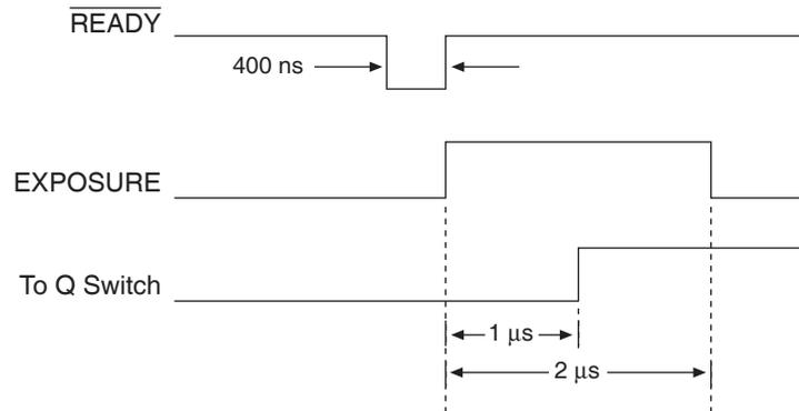
Figure 53. Timing for Experiment Setup shown in Figure 52
