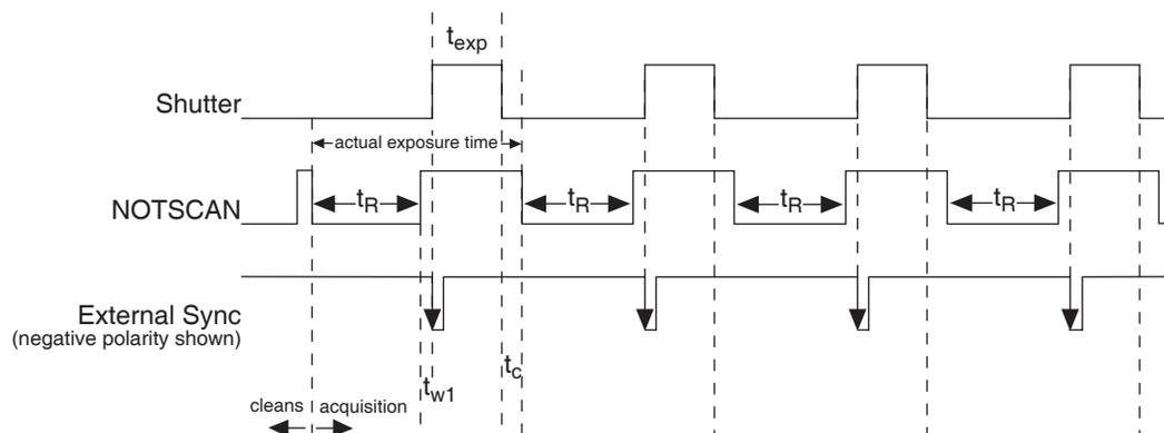
Figure 46. Overlapped Mode where Pulse arrives after Readout
