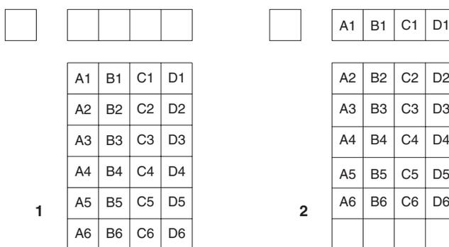
After the first row is moved into the shift register, the charge now in the shift register is shifted toward the output node, located at one end of the shift register. As each value is "emptied" into this node it is digitized. Only after all pixels in the first row are digitized is the second row moved into the shift register. The order of shifting in our example is therefore A1, B1, C1, D1, A2, B2, C2, D2, A3....
