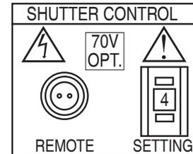
Figure 2. ST-133 Rear Panel with 70 V Shutter Option
