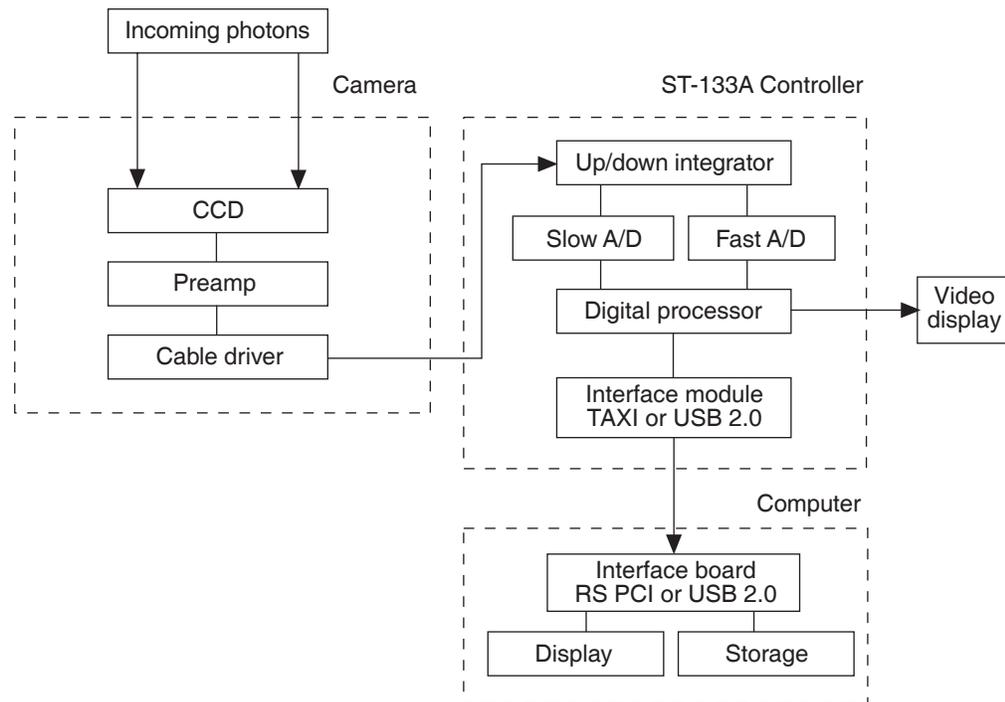
Figure 25. Block Diagram of Light Path in System
