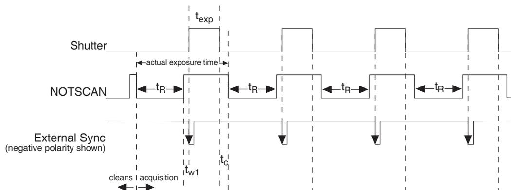
Figure 18. Frame Transfer where Pulse arrives after Readout
