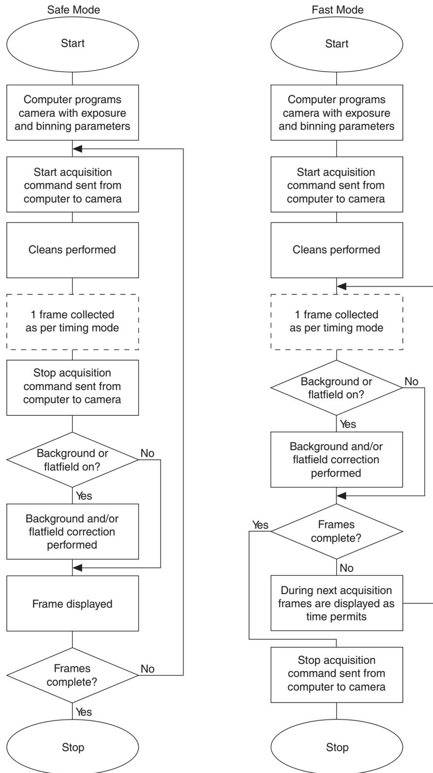
Figure 9. Flowcharts of Safe and Fast Mode Operations
