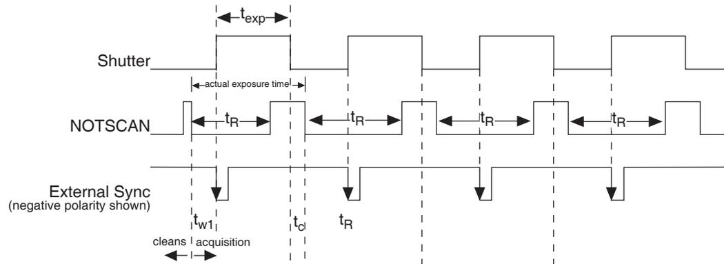
Figure 17. Frame Transfer where  $t_{w1} + t_{exp} + t_c > t_R$
