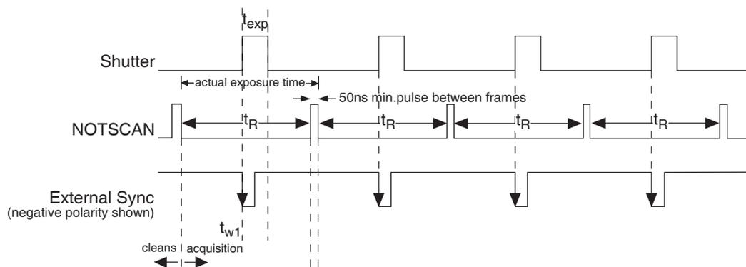
Figure 16. Frame Transfer where  $t_{w1} + t_{exp} + t_c < t_R$
