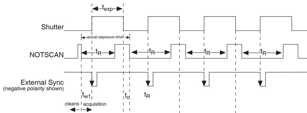
Figure 45. Overlapped Mode where  $t_{w1} + t_{exp} + t_c > t_R$
