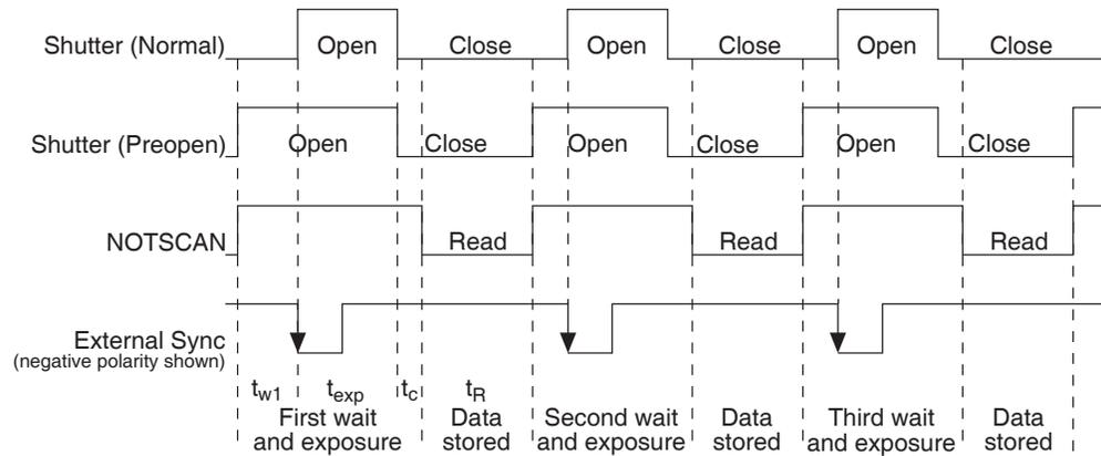
Figure 13. Timing Diagram for the External Sync Mode
