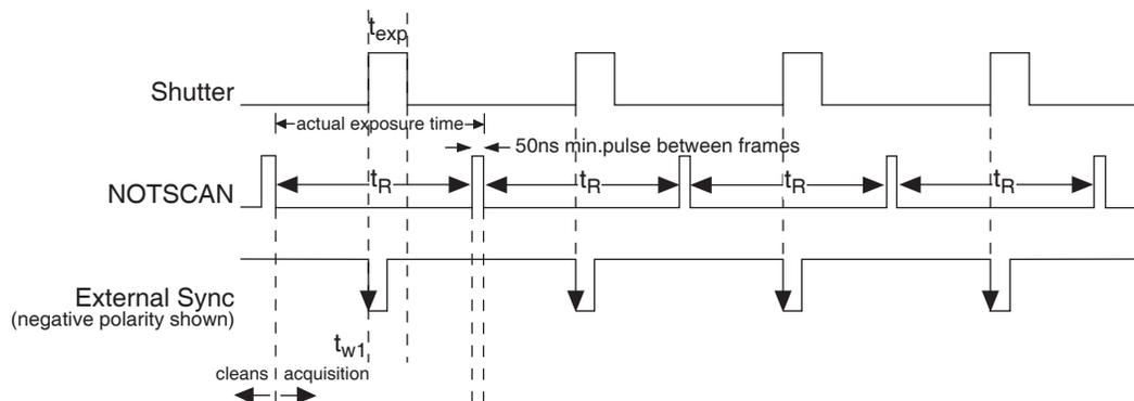
Figure 44. Overlapped Mode where  $t_{w1} + t_{exp} + t_c < t_R$
