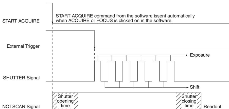
Figure 23. Single Trigger Timing Diagram
