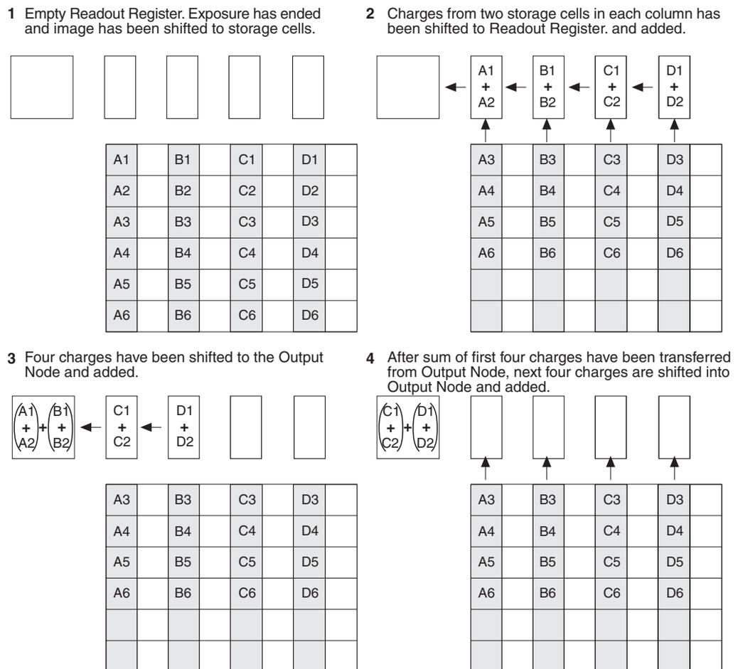
Figure 50.  $2 \times 2$  Binning for Images
