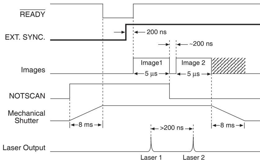
Figure 54. Timing Diagram for Typical IEC Measurement
