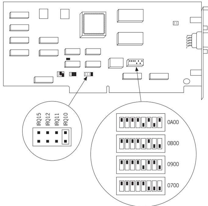
Figure 61. ISA Board Switch and Jumper Settings
