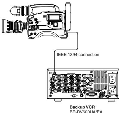
When this unit is connected to a DV camcorder (GY-DV500/DV550) via the IEEE 1394, a long-time recording is possible by starting recording in this unit around the time after the recording tape in the source VCR ends.
